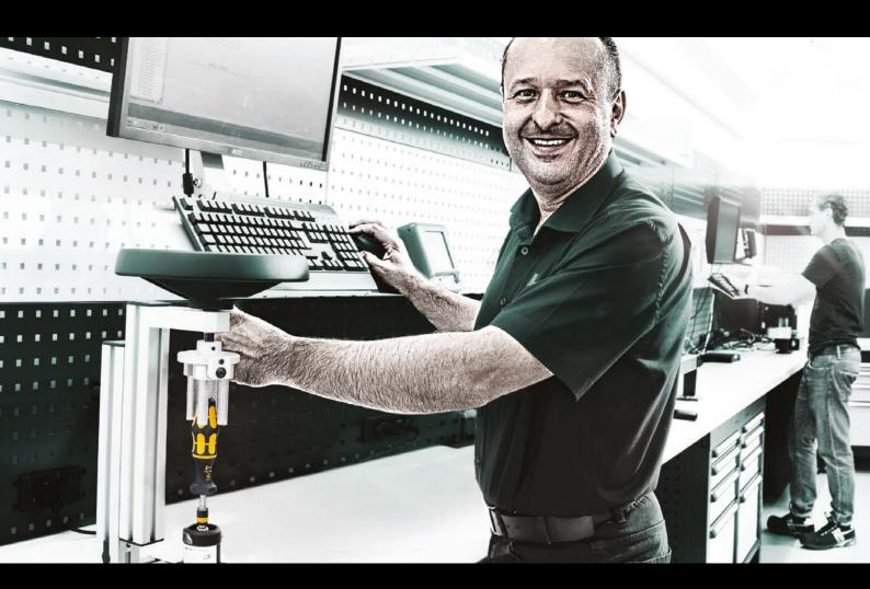
All Wera torque tools are produced, adjusted, calibrated and certified under strict quality conditions. On request, Wera can also issue a calibration certificate according to DAkkS standard in cooperation with an accredited specialist laboratory.
