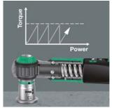
The Safe-Torque torque wrench is equipped with a slide-over mechanism. Once the set torque value has been reached, the tool cannot be overtightened, so that excessive torque cannot be applied.
