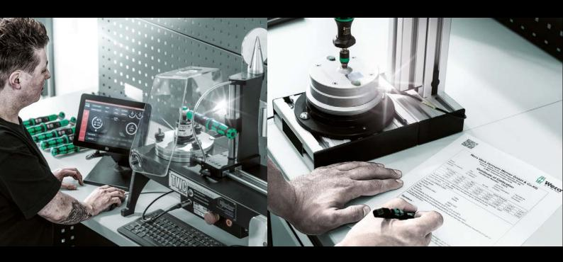
As part of our service packages, we offer you not only calibration and, if necessary, the adjustment of your torque tool, but also the repair or replacement of defective components.
