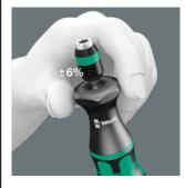
These torque screwdrivers are supplied with a fixed pre-set torque value. This is ideal for all applications that require constant, identical torque. They feature a pre-set torque range of 0.3 Nm to 4.0 Nm (adjustable between 0.3 Nm - 8.8 Nm), two different handles, measurement accuracy of ± 6 % and Rapidaptor chuck
