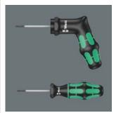
Wera torque-indicators have been factory pre-set to values recommended by leading carbide tool manufacturers. These tightening values relate specifically to the size of the TORX®, TORX PLUS® or hexagon socket screw. Torque indicators ensure safe and easy loosening of screw connections. Precision: ± 10 %.
